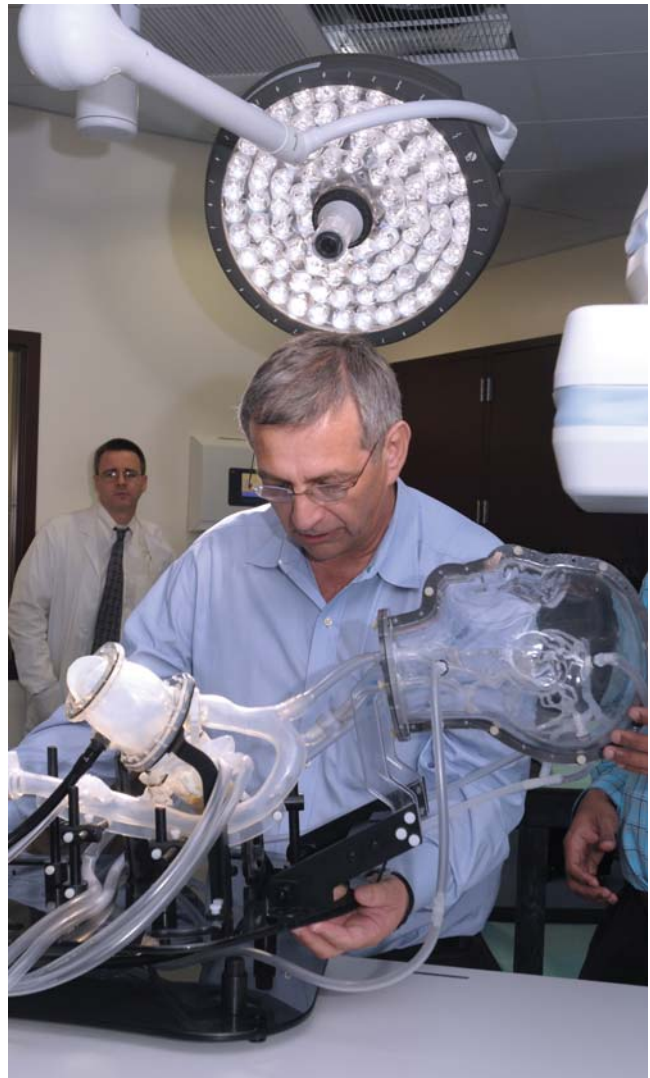
Affectionately known as “Headley,” the neuroendovascular simulator is supported by the only robotically powered multi-axis angiography imaging technology in the region dedicated solely to research, and some of the region’s most sophisticated imaging technology.
